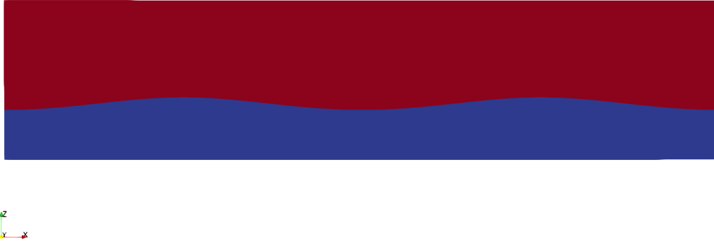
FIGURE 12. Numerical results of liquefaction criteria after 15 minutes of Example 2 (exaggerated z -axis). The red and blue colors indicate the liquefied and non-liquefied regions, respectively.
